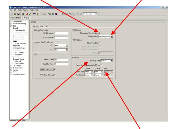
Change the Power up State to T-Mode so that when the radio powers up it starts up in Transparent Data mode.
